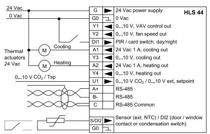
The maximum triac output current is 1 A. For example, up to four A4004 thermal actuators can be connected to one output. Then the total current consumption doesn't exceed 1 A.
