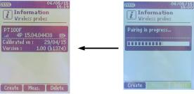
The probe information is displayed With the function key "Meas." It is possible to back to the measurement screen. It is also possible to delete the wireless probe pressing the function key "Delete".
