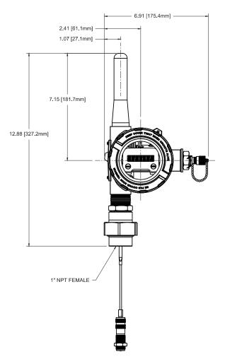
2.4GHz INTEGRAL ANTENNA AND CABLED ANTENNA OPTIONS
