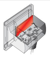
The general purpose non-intrusive capacitance level switch provides reliable liquid level detection of water based conductive liquids with non-coating and/or scaling characteristics with a 1A relay output. Media examples include hydrochloric, sulfuric acid and water. The liquid level sensor is bracket mounted on the exterior wall of non-metallic tanks and applied as a high level alarm or low level alarm.
