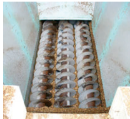
Mounting in discharge screw (wood-fired power plant)
