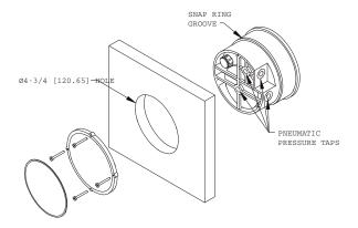
A. PANEL MOUNTING: Cut a 4-3/4" or 120mm dia. hole in panel and insert the complete unit from the front. Slip on the mounting ring and install the split snap ring in the groove on the bezel. Seat the mounting ring against the snap ring and thread the four screws through the tapped holes. Tighten screws against rear of panel.
