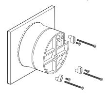
C. FOR -SS BEZEL INSTALLATION: Provide a 4-9/16" opening in panel. Insert gage and secure with supplied mounting hardware.
