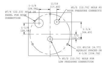
MOUNTING: The Photohelic® Switch/Gage may be either panel mounted or surface mounted.
