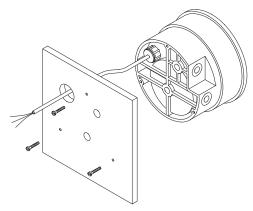
B. SURFACE MOUNTING: Drill (3) 3/16" dia. holes for mounting screws and (1) 7/8" dia. hole for wire assembly as shown in hole location drawing. Insert screws from rear of panel and thread into tapped holes on back of Photohelic® Switch/Gage case. If rear pressure connections are to be used, make 1/2" dia. holes located as shown in hole location drawing in left column.
