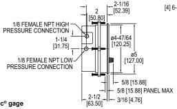
[4] 6-32 HOLES EQUALLY SPACED ON A 5-1/8 [130.18] B.C. ø4 [101.60] FACE 5-1/2 [139.70]
