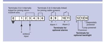
Output Isolated solid state switch complying with requirements for simple apparatus.
