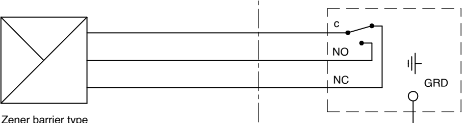
Fig. 6: Operation of pressure switches in intrinsically safe areas
