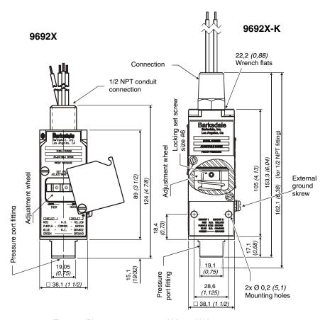
Fig. 8: Piston sensor type 9692X / 9692X-K
