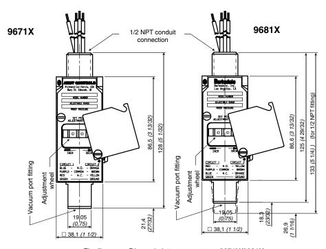
Fig. 7: Dia-seal piston sensor type 9671X/9681X
